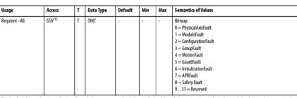
The Axis Fault Bits attribute is a collection of basic fault types associated with the axis. Each valid axis fault type is assigned a bit in this word. Any fault condition associated with a given fault type will result in the setting of the appropriate axis fault bit.
